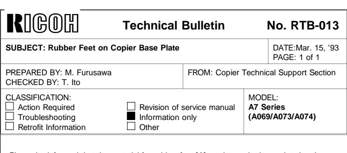
Please be informed that the material for rubber feet [A] on the copier base plate has been changed from hard rubber to molding since June, 1992.
